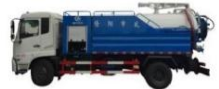
DONGFENG sewer dredging vehicle, 4m 3 water tank and 4.5m 3 sewage tank, 180hp, cummins engine
