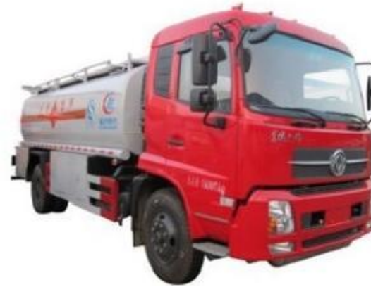
Dongfeng 4x2 chassis,180 hp, 12-15cbm fuel tank,fuel tank truck
